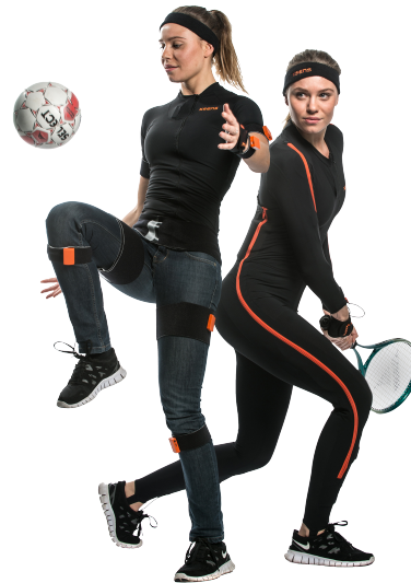
Fig. 1. Xsens MVN consists of 17 inertial and magnetic motion trackers. Data from wireless ( MVN Awinda ) or wired ( MVN Link ) trackers is transmitted by a wireless connection to a PC where the data is further processed and visualized.
